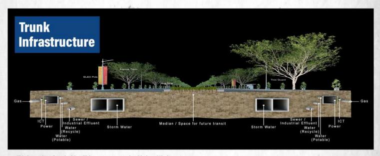
This is section of road with utilities as constructed at Dholera SIR site.
