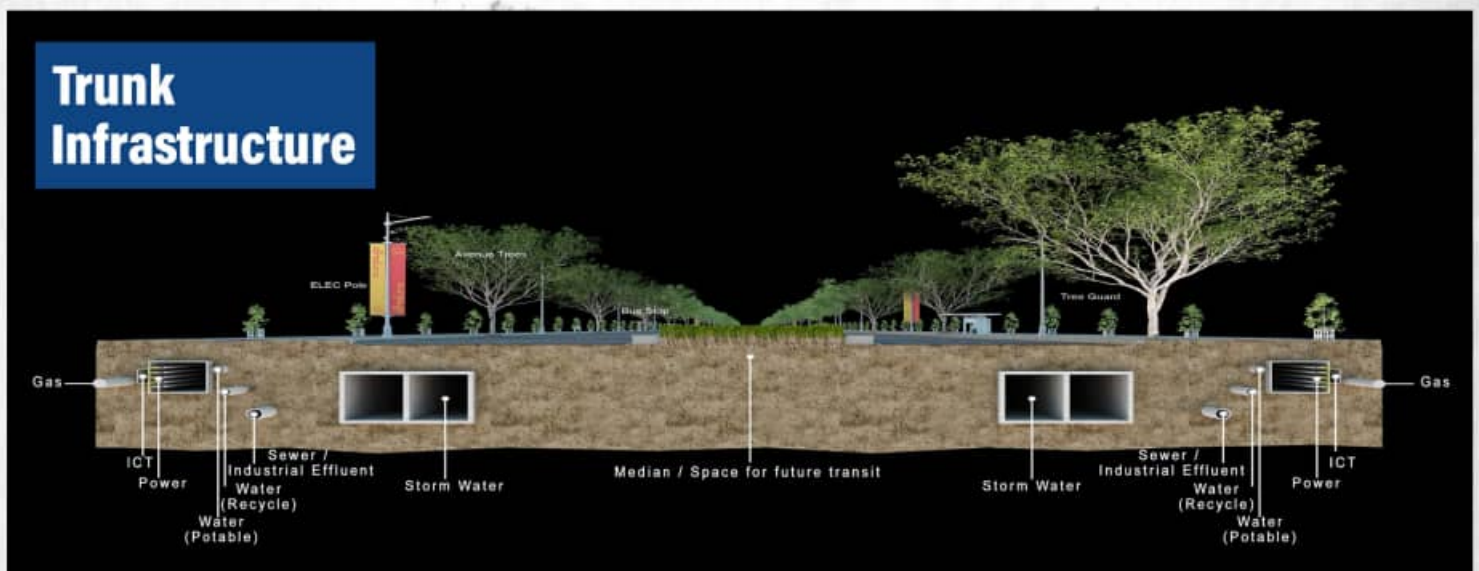
This is section of road with utilities as constructed at Dholera SIR site.
